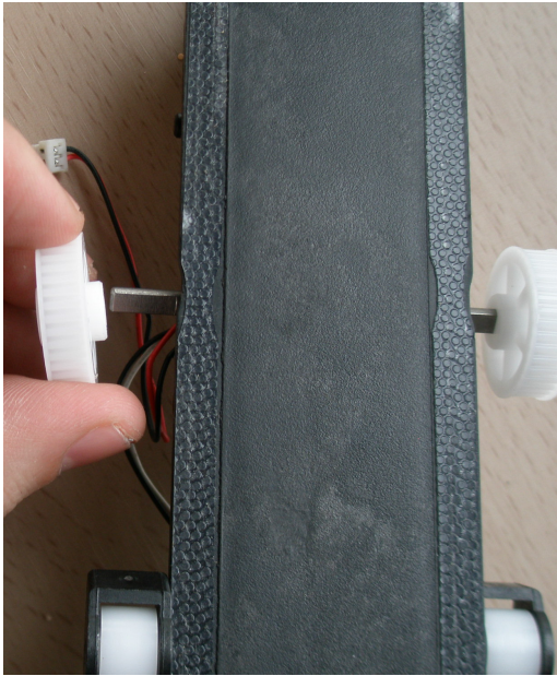
Remove wheels of both sides of Gearbox.
